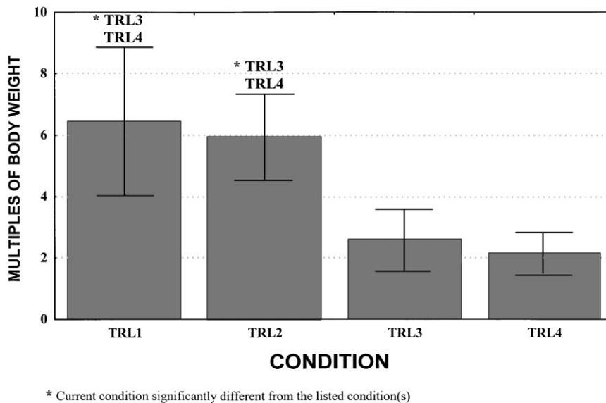
Fig. 6. Average impact force ( $\pm$  S.D.), in multiples of body weight, for the box trailer. Significant paired post-hoc comparisons are also indicated. Refer to Table 1 for description of the conditions.
