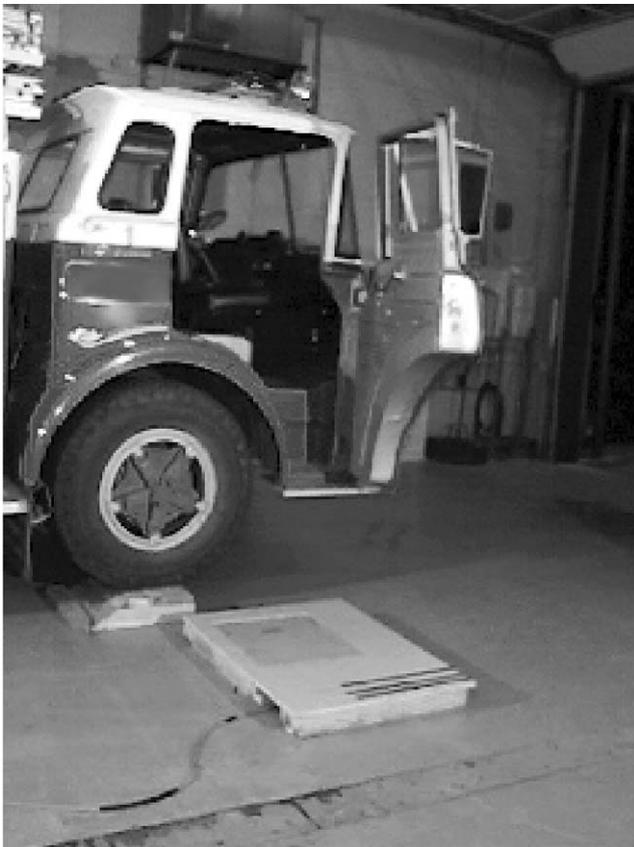
Fig. 8. Vertical impact force measurement set-up in fire station "B": the pumper is driven up on wooden ramps having the same height as the force platform, seen here embedded in a false floor.
