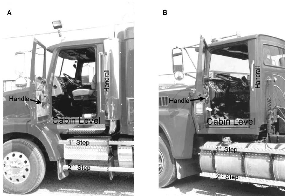
Fig. 1. Illustrations of the cabins used in this study: (A) Western Star 98 (WS) and (B) Ford 9000 (F9K).
